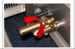
Unscrew the air valve and remove it from the tap.
