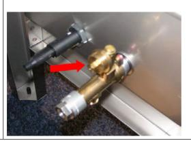
Replace the fuel injector with the specimen supplied along with the equipment.
